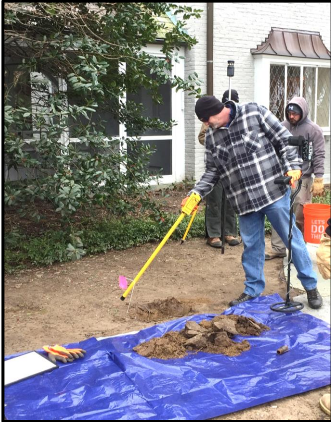
Checking a excavation location with a Schonstedt & Whites metal detector to ensure the metal anomaly was removed
